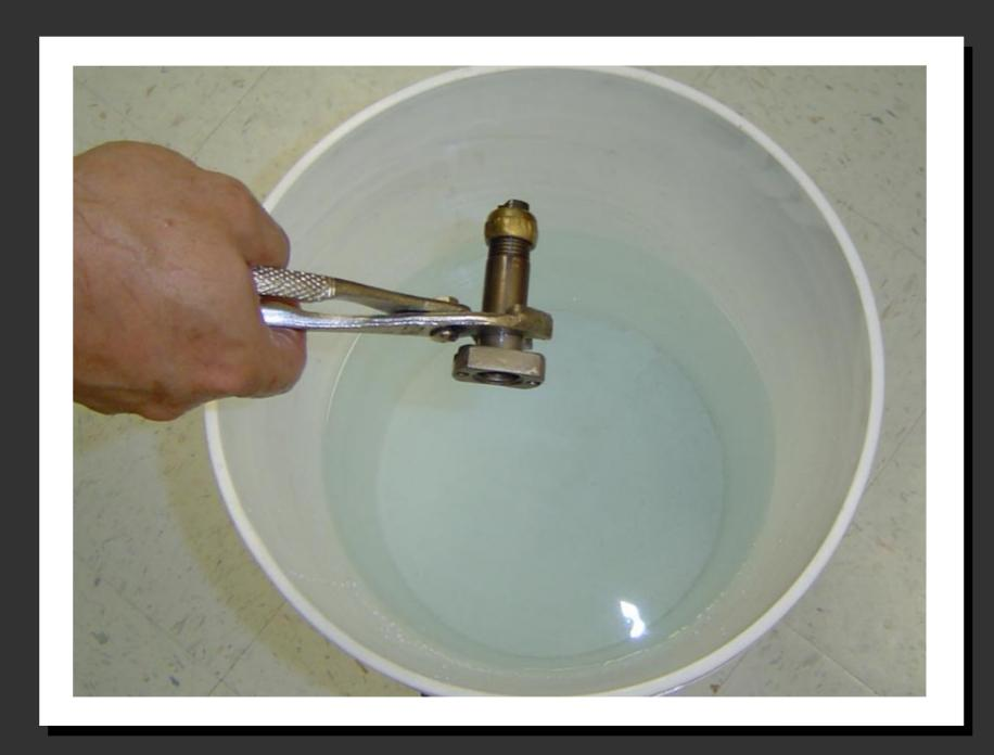
Cleaned part being quenched in a bucket of water
