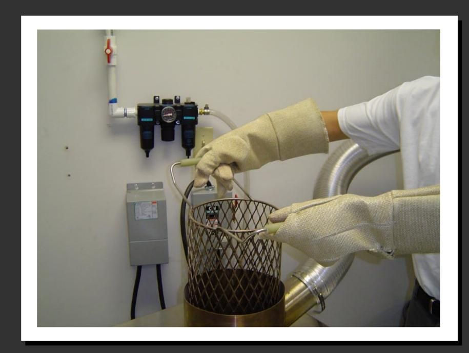
Remove the hot basket with cleaned part, safety first
