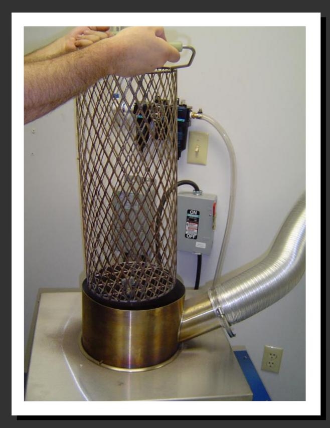
Insert the basket with part into the bath at temperature
